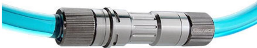
QDC shutoffs work by having an internal valve that self-seals and opens as needed. Both male and female fittings contain a "plunger" that is spring-activated. When connected, the valves on both sides remain open to allow coolant to pass through. When detached, each side immediately closes.
