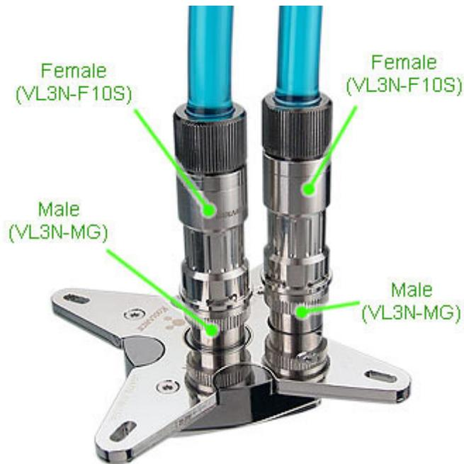
You will need one male and one female fitting for any hose you wish to disconnect. To detach two hoses (inlet/outlet) going to a water block or pump, you would need two male and two female QDC. So long as Koolance fittings are selected from the same series, any male will connect to any female fitting.
